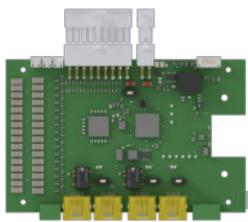
Each Solar MD battery, whether low or high voltage, has its own Battery Management System (BMS) designed and built in-house. The BMS handles the internal functions of each battery.
