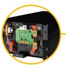
Additional the combiner box has a mounting space for the Logger V2 and connects all communication cables between batteries and Logger.
