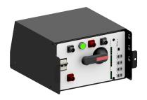
The BMU is used in combination with the SS6143 modules and forms part of our high-voltage energy system. It is responsible for gathering data from the entire battery system, performing state of charge (SOC) calculations, and facilitating information exchange among the various battery modules in its cluster.
